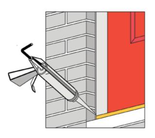
NB: Care must be taken to ensure that the drainage slots are not blocked when sealing around the aluminium wheelchair threshold.
