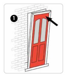
Offer complete door unit into brickwork opening.
