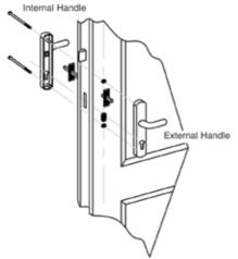
NB: When the door has been fixed into position the operation of the door opening and locking mechanism must be checked to ensure uniform contact with weatherseals and correct function of handle/lock.
