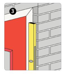
Spirit level (1.5m Long) should be used to ensure jambs are square and plumb in all planes.
